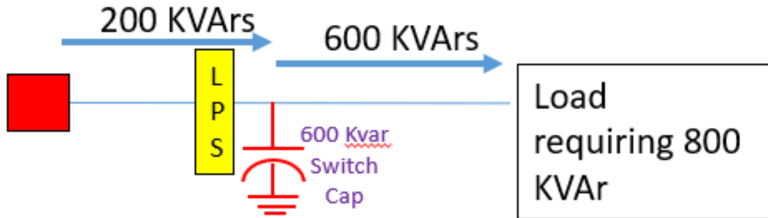
Linepost Sensor mounted on Source Side of Capacitor Bank
